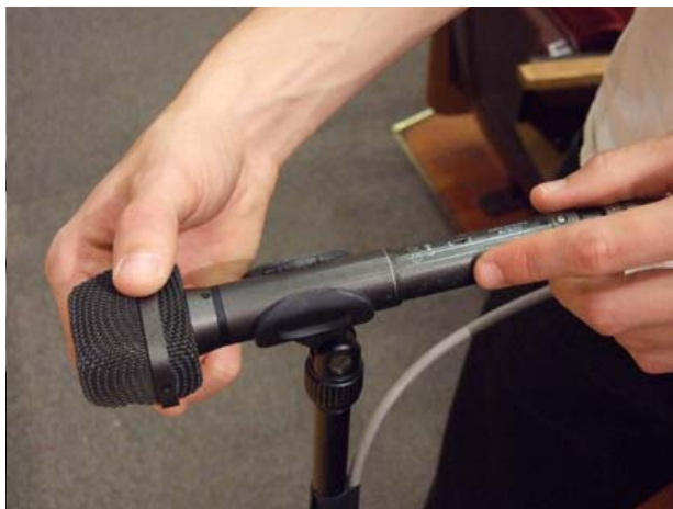
Make certain the the microphone is right-side up. The lettering is on top.
