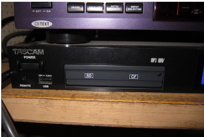
Tascam uses USB, SDHC or CF memory devices.
