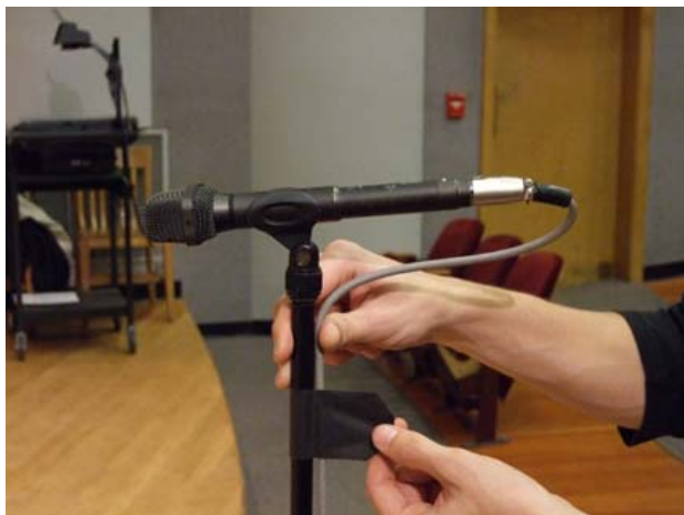
Some tape can help hold the cable and prevent the microphone from tipping back.
